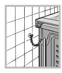
!Some models can have their gas connection inverted. It is important to make sure the safety chain is always situated on the side which corresponds to the hose holder (Fig. B).
